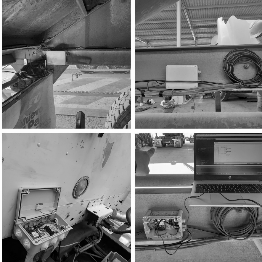
Fig. 5. Tests for IoT Node Station prototype attached to a cargo truck.
